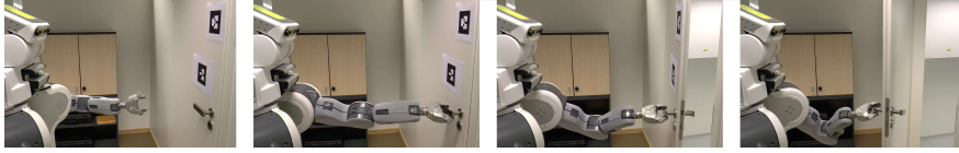
Fig. 7 The resulting motion after learning the door opening task is depicted in this slideshow. See Section 5.3 for more details.
