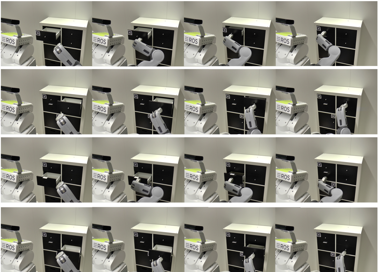
Figure 13. Resulting motions of the drawer closing experiments with the PR2 (see Section 6.6). We used two demonstrations for different drawers as input for our inverse KKT method. Each row shows a resulting motion after optimizing the cost function for a different drawer of the shelf.
