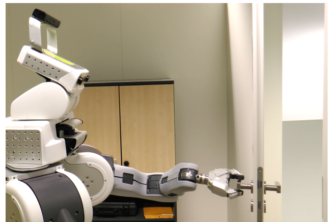
Figure 1. This picture shows the door opening task that we use to evaluate our approach by first learning a cost function from demonstration and then generating motions by optimizing the cost function for different scenarios (e.g., initial positions, door angles). See Section 6.5 for more details.
